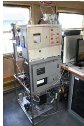
Apparatus for RHR measurement ( O_2 -CO-CO 2 )
