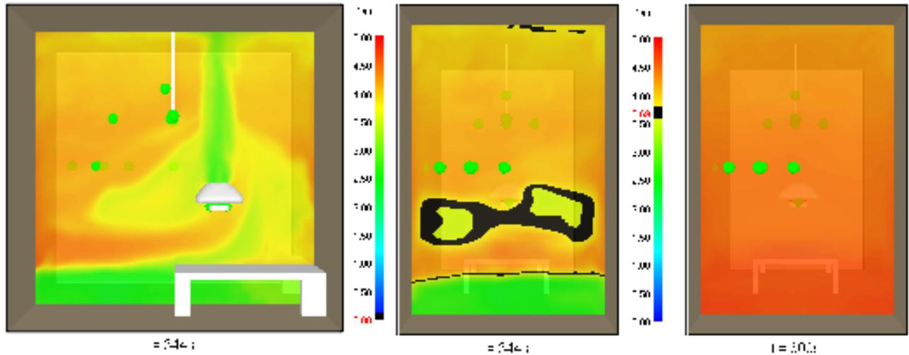
**Figure 3:** Smoke visibility after 344 and 600 seconds with 1cm grid resolution
