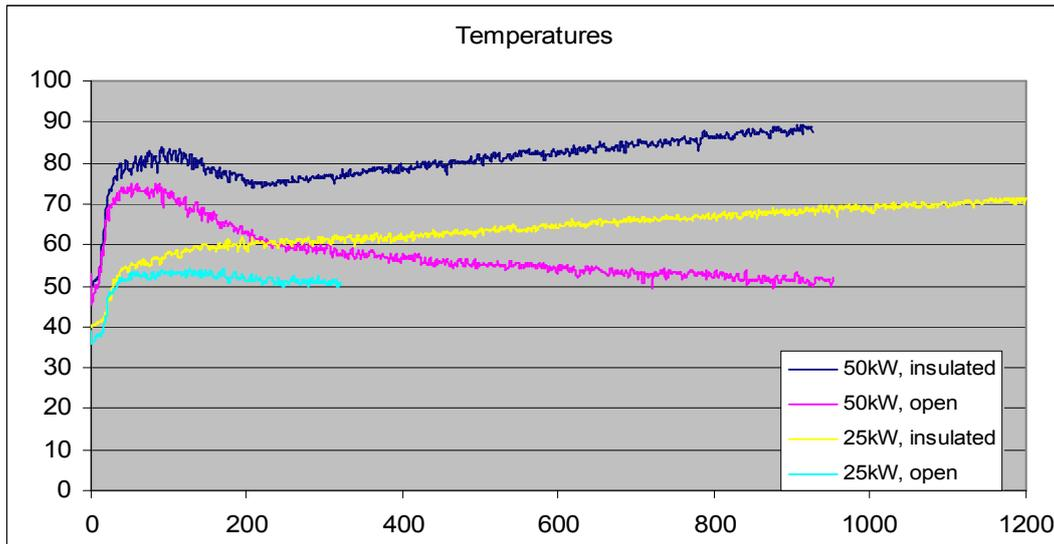
**Figure 1:** The temperature in the middle of the chamber with different boundary conditions
