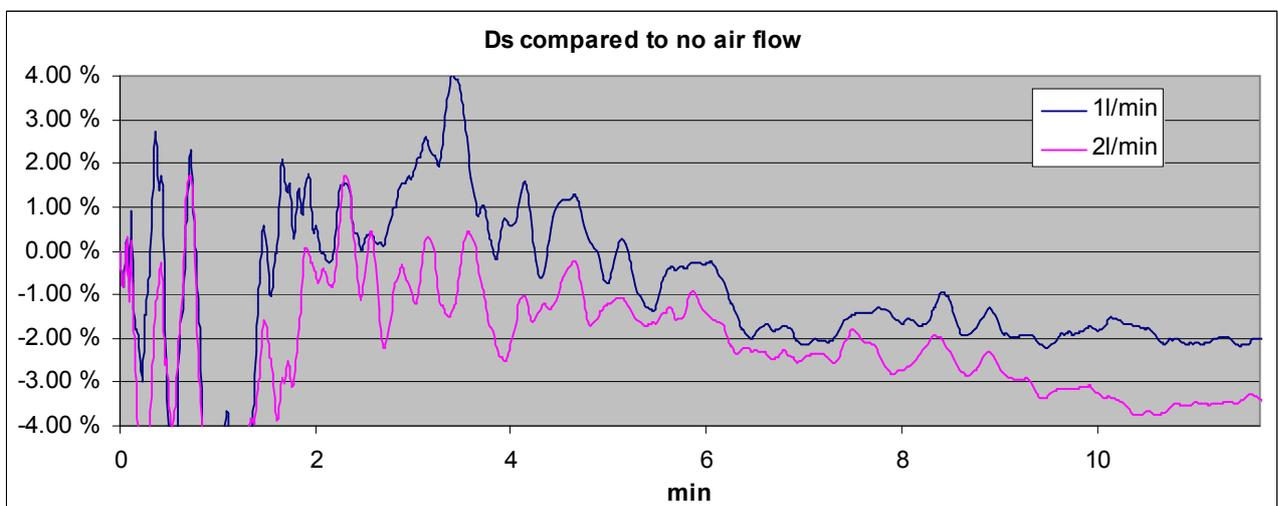
**Figure 8:** Ds difference with different sampling probe air flow rates
