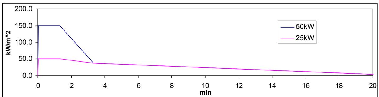
**Figure 12:** Specimen heat release rates as a function of time
