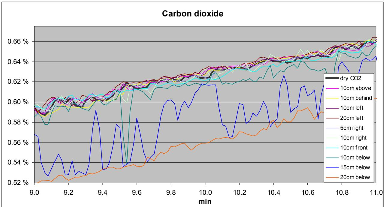
**Figure 6:** CO<sub>2</sub> concentration as a function of position relative to the sampling point with 1 cm and 2 cm mixed grid resolution, 25 kW heat flux and insulated walls
