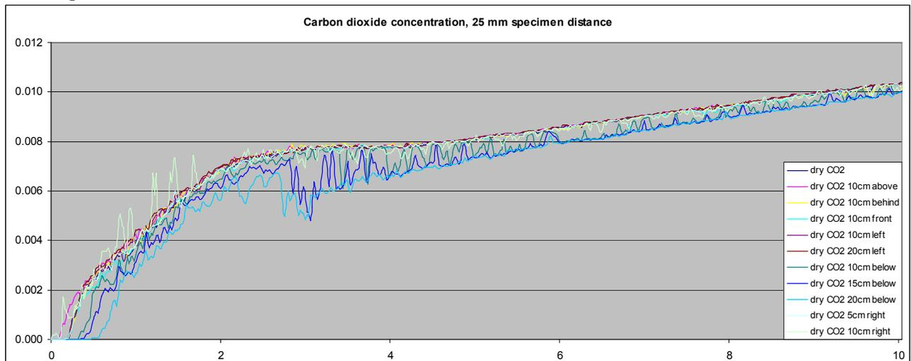
**Figure 10:** Carbon dioxide concentrations with 25 mm specimen distance
