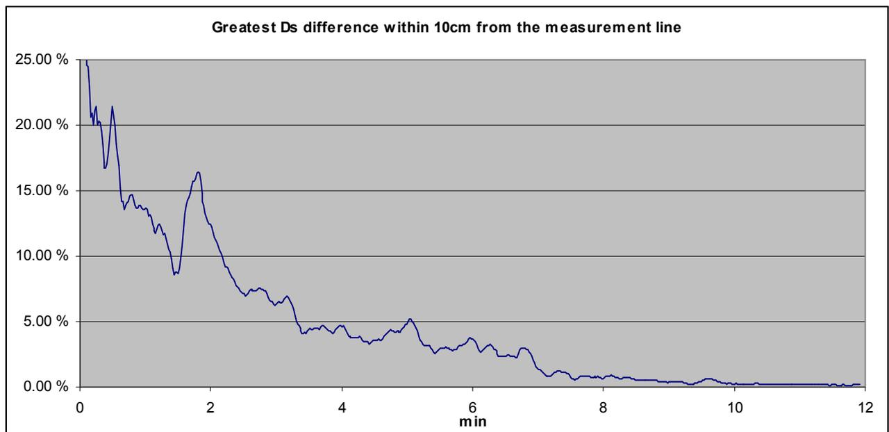
**Figure 4:** Greatest  $D_s$  difference with 1cm grid resolution, 50 kW heat flux and insulated walls
