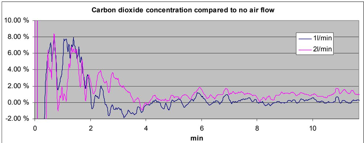
**Figure 9:** Carbon dioxide concentration difference with different sampling probe air flow rates
