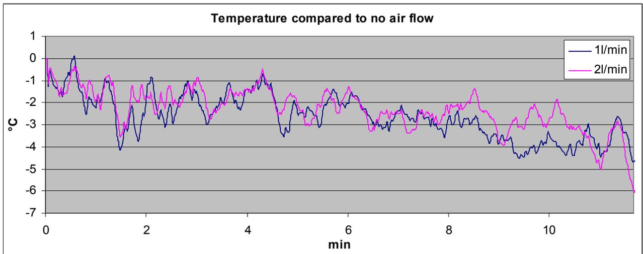
**Figure 7:** Sampling temperature difference with different sampling probe air flow rates
