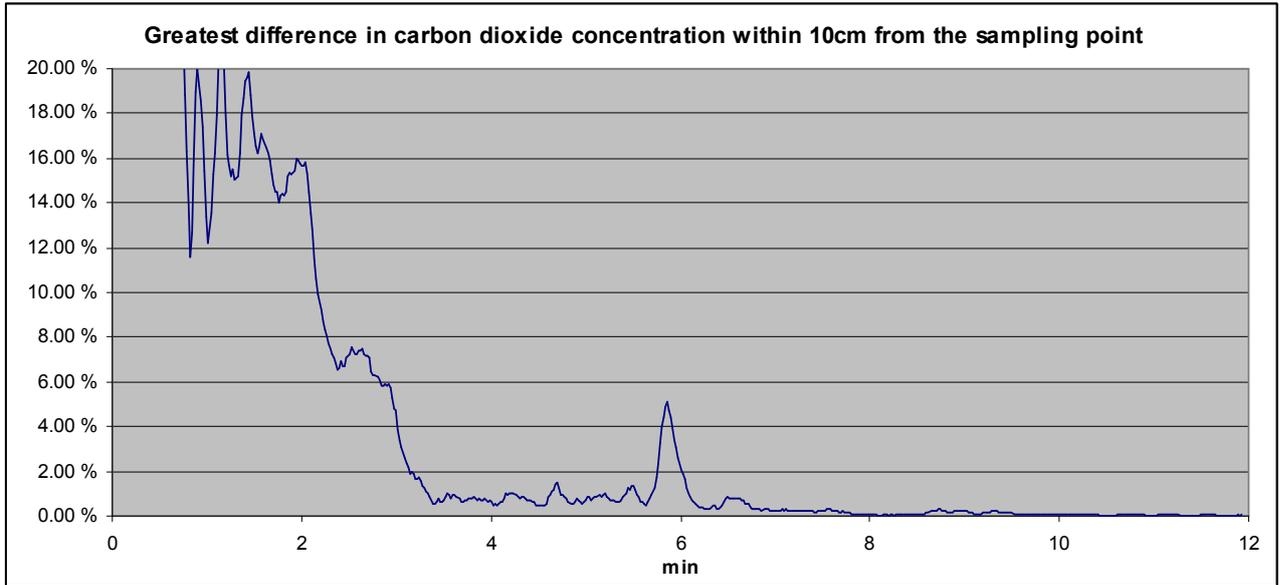
**Figure 5:** Greatest difference in CO<sub>2</sub> concentration with 1cm grid resolution, 50 kW heat flux and insulated walls
