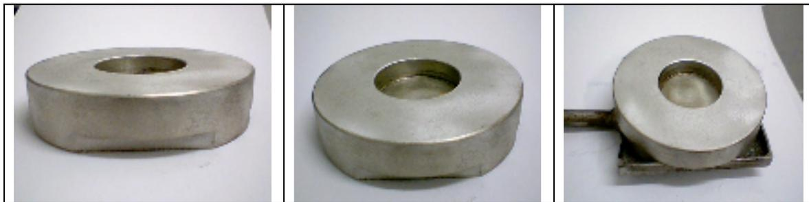
The small crucible tank shall be placed in the central hole and the exceeding part shall be covered by a non combustible calcium silicate pad as shown in the following picture.
